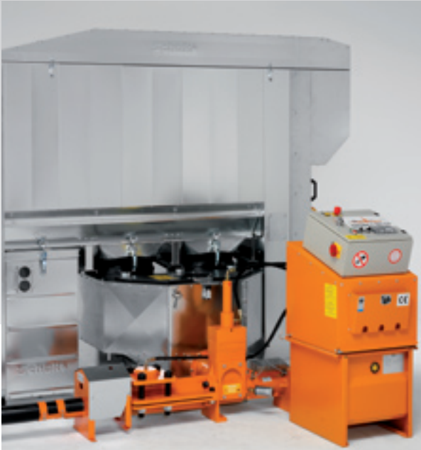
Briquetting press Compacto 800 in front of VACOMAT 200 deduster and SPB 40 chip container
