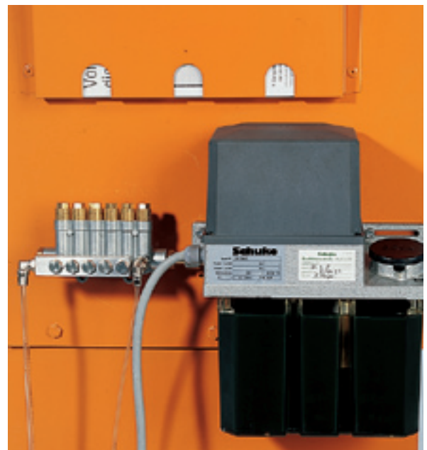
Central lubrication system for automatic lubrication of the briquetting press (not included in scope of delivery)
